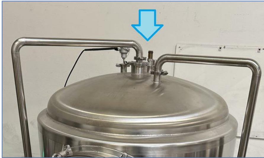
Figure 22 – Valves on Top of Blue Myco Pressure Cooker Dome
