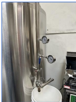
Figure 9a - Blowoff Arm (Left) and Figure 9b - Adjustable 14.7PRV connected to the Butterfly Valve (Inside Bucket; Right)
