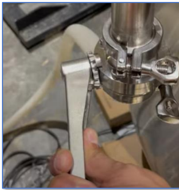
Figure 23 – Butterfly Handle Correctly Positioned and Venting Hose Hooked Up
