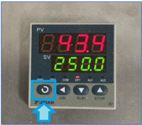
Figure 25a – Menu Button on Left Hand Side (Left) and Figure 25b – Menu Choice to Put in Passcode (Right)
