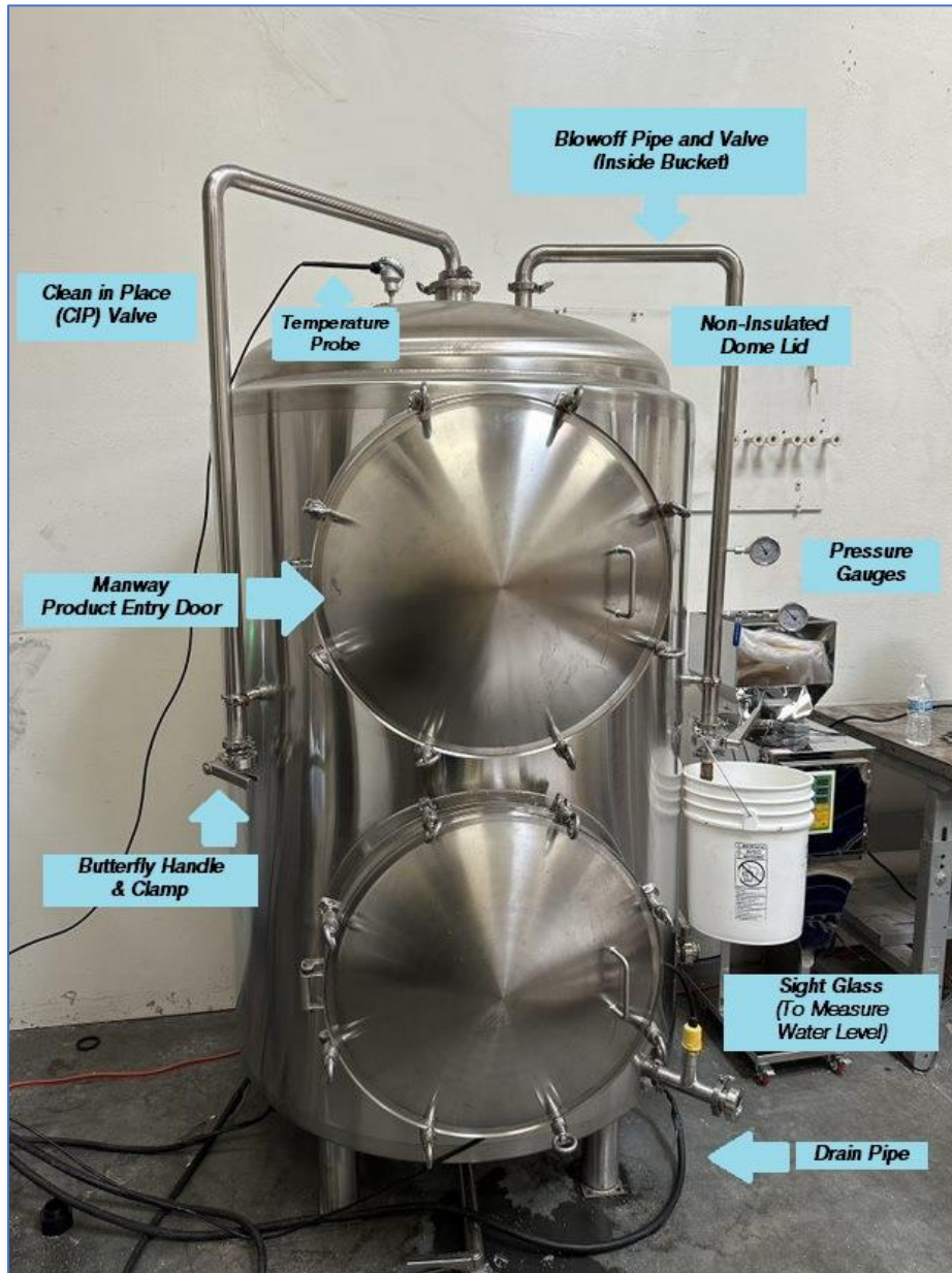
Figure 1 – Blue Myco Pressure Cooker Main Components
