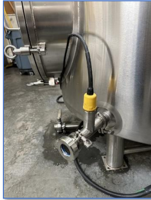
Figure 10 – Water Level Sight Glass Indicator
