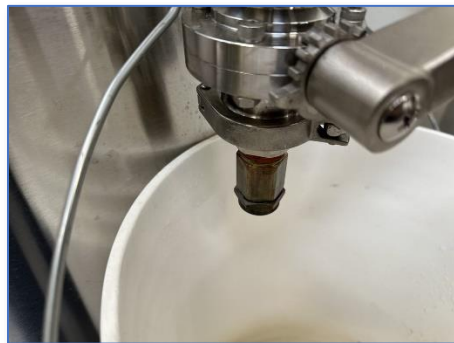
Figure 9a - Blowoff Arm (Left) and Figure 9b - Adjustable 14.7PRV connected to the Butterfly Valve (Inside Bucket; Right)
