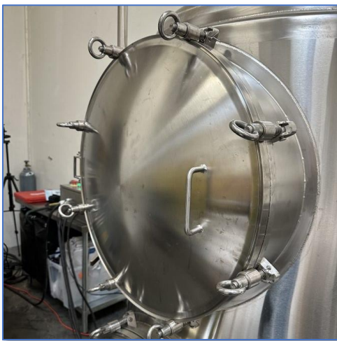
Figure 7a – Manway w/Clamps (Left) and Figure 7b – Manway Opened with Product in Vessel
