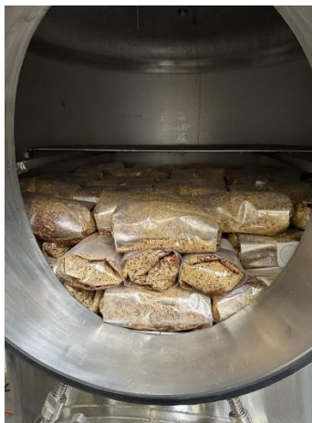
Figure 20 – Example of Properly Staged Product Inside Vessel
