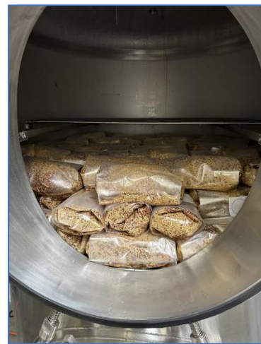
Figure 7a – Manway w/Clamps (Left) and Figure 7b – Manway Opened with Product in Vessel
