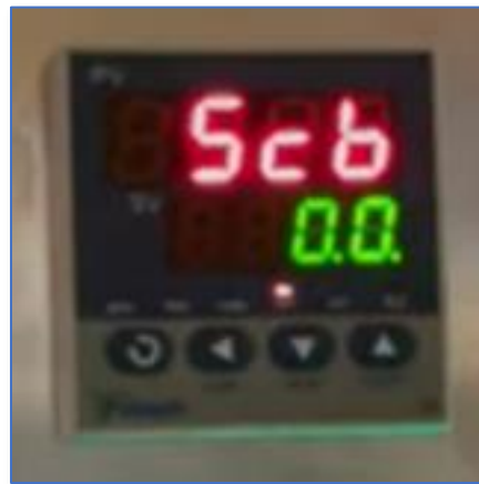
Figure 27 – 'Scb' Menu Option on Temperature Readout
