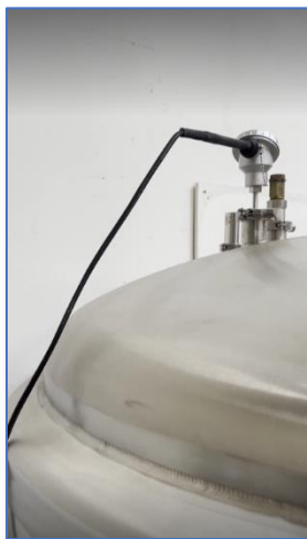
Figure 4 – Temperature Probe (Left) and Figure 5 – Pressure Release Valve (PRV) (Right)
